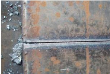
Sample of steel plate cut by flame cutter.
